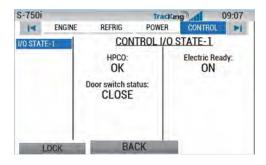
I/O State-1: Displays information for High Pressure Cutout (HPCO), Electric Ready Input, Door Switch Status.
