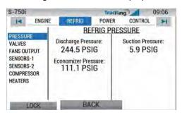
Pressure: Displays the Compressor Discharge Pressure, Compressor Suction Pressure, Economizer Pressure.
