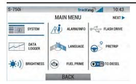
The basic system information will be displayed on the System submenu. This is information deemed critical/important to the user. Press the UP and DOWN keys to scroll through the system information. Selecting the LOCK key will lock the current system information on the display. Selecting the LEGAL key will display the Legal Disclaimer QR Code.
