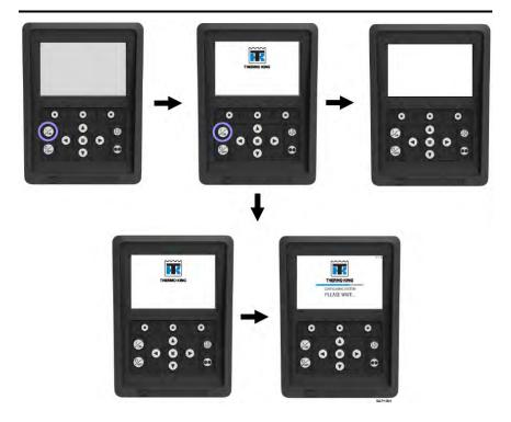
Once the system startup sequence is completed, the Standard Display will appear and the unit will start in Diesel Mode (if no Electric Standby is detected). The temperature setpoint or other system changes can now be made if required.
