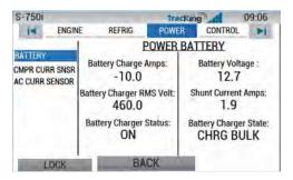
Battery: Displays Battery Charge Amps (Amps flowing to or from the unit battery), Battery Voltage, Battery Charger Input Voltage (RMS Volts), Shunt Current (Amps consumed by control system), Battery Charger Status, Battery Charger State.
