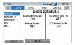
ECU Input-1: Displays the current state of the following inputs: Engine Starter Command Low Side and High Side, Preheat Enable, ECU Power Enable.
