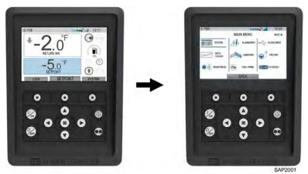
Figure 14. Standard Display and Main Menu Display
