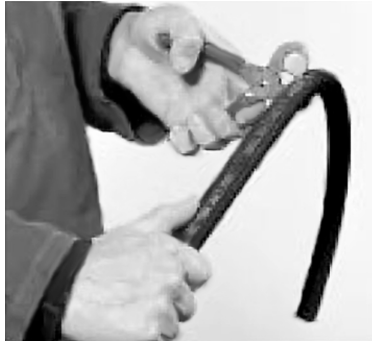
Figure 54. Cut the hose with an appropriate cutting tool.
