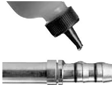
Figure 56. Apply oil to the nipple and both O-Rings.
