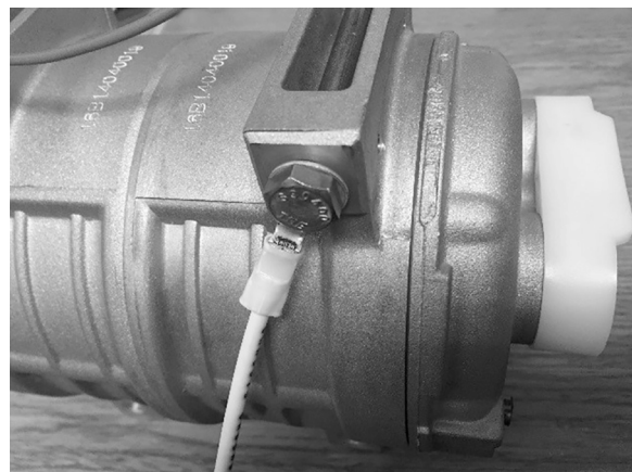
Ground Strap shown installed on ear mount style and direct mount style compressors.
