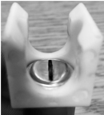
Figure 38. Sensing pad and plastic clip shown perfectly aligned.
