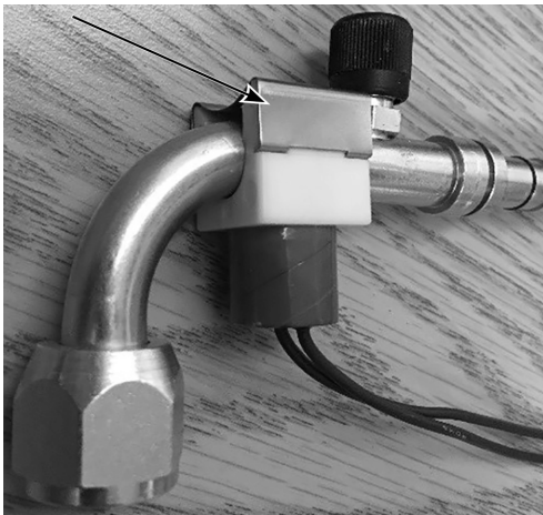
Figure 41. Spring clip shown correctly installed.
