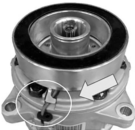
Figure 35. Clutch Coil Installed and Wires Properly Routed.
