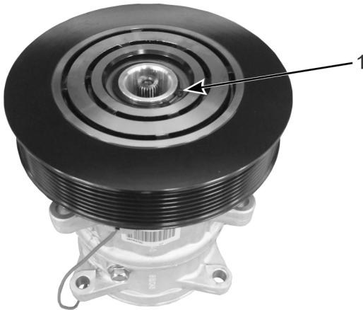
Figure 36. Install Pulley and Snap Ring.
