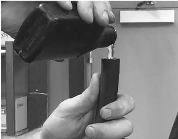
Figure 25. Add oil into suction line.
