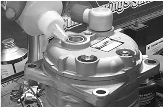
Figure 22. Add oil to O-rings.
