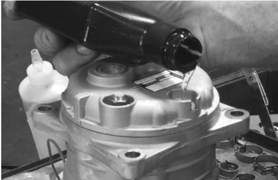
Figure 21. Add oil to compressor.
